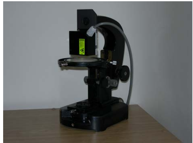
Figure 2. Picture of the microdisplacements measuring device
